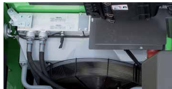
The large reversing fan provides up to 45% more of the cooling surface than comparable machines.
