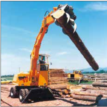
1974: Timber handling machine with elevated cab
