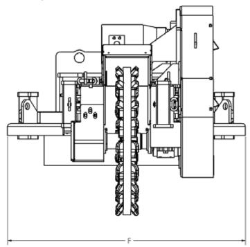
The stump grinder attachment is available for the C250, C400L and C450. Equipped with a 38 inches diameter Bucktooth<sup>®</sup> wheel, it has a greater torque than the competition. The 64 teeth on the wheel make a smoother cut.
