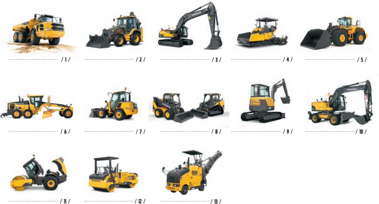
1 / Articulated haulers // 2 / Backhoe loaders // 3 / Crawler excavators // 4 / Pavers // 5 / Wheel loaders // 6 / Motor graders // 7 / Compact wheel loaders // 8 / Skidsteer loaders // 9 / Compact excavators // 10 / Wheeled excavators // 11 / Soil compactors // 12 / Asphalt compactors // B / Milling machines
