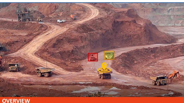
**SAFEYE** is an advanced stereoscopic machine vision system that detects differentiates between pedestrians, industrial machines like dump trucks, excavators, forklifts, cars, and other machines typically found on industrial sites.
